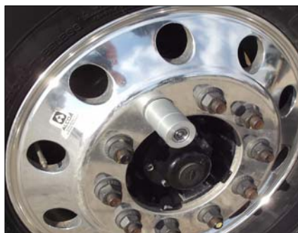
Dealer lot security version features heavy duty lock-only unit. No chrome cover.
