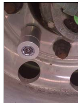
Dealer lot security version features heavy duty lock-only unit. No chrome cover.
