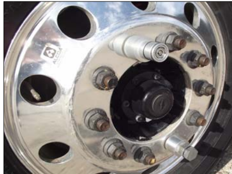
Counter-weight that maintains wheel balance.
